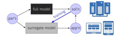
Process data coming from **expensive** simulations to build a **cheap** surrogate model that can give **useful** information, with **"enough" accuracy**
